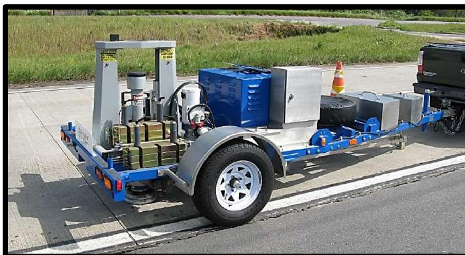
Figura 30. Falling Weight Deflectometer. Fuente: [www.thetranstecgroup.com](http://www.thetranstecgroup.com)
