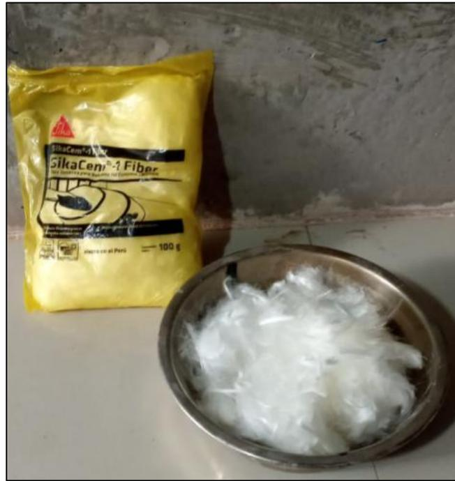
Figura 24: *Fibras SikaCem – 1 Fiber*
