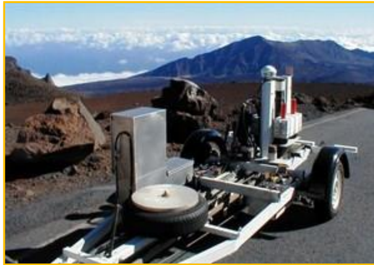
FIGURA N° 29: FALLING WEIGHT DEFLECTOMETER (FWD)
