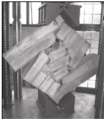
Figura 26 falla semi diagonal
